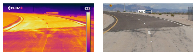
Figure 14: The light color of concrete pavement reduces surface temperatures and mitigates UHI impacts
